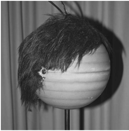
FIG. 9. Experimental setup showing the wooden sphere with the synthetic hair covering. The hairline is elevated 45^\circ and the microphone (ear) is set within the azimuth plane, offset from the frontal median axis by 90^\circ .
