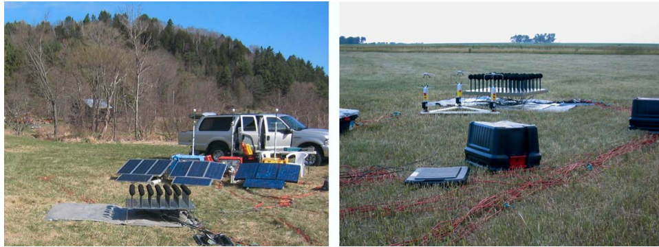
Fig. 1. (Color online). Left: W. Fairlee, VT site, showing the microphone array and solar panels. Right: Tolono, IL site, showing the microphone array and ultrasonic anemometers.
